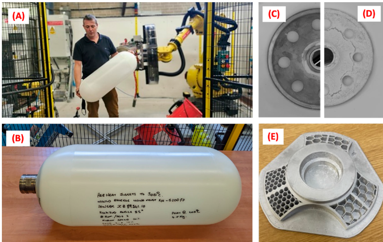
Figure 8. (a) Liner molded using electronically heated rotational molding tool, (b) Example of a single ended tank liner with a boss, (c) Boss acting as a heat sink resulting in poor encapsulation, (d) Onset of encapsulation on the inside face of a boss, (e) Part of a Metal Printed Boss Prior to Molding.
