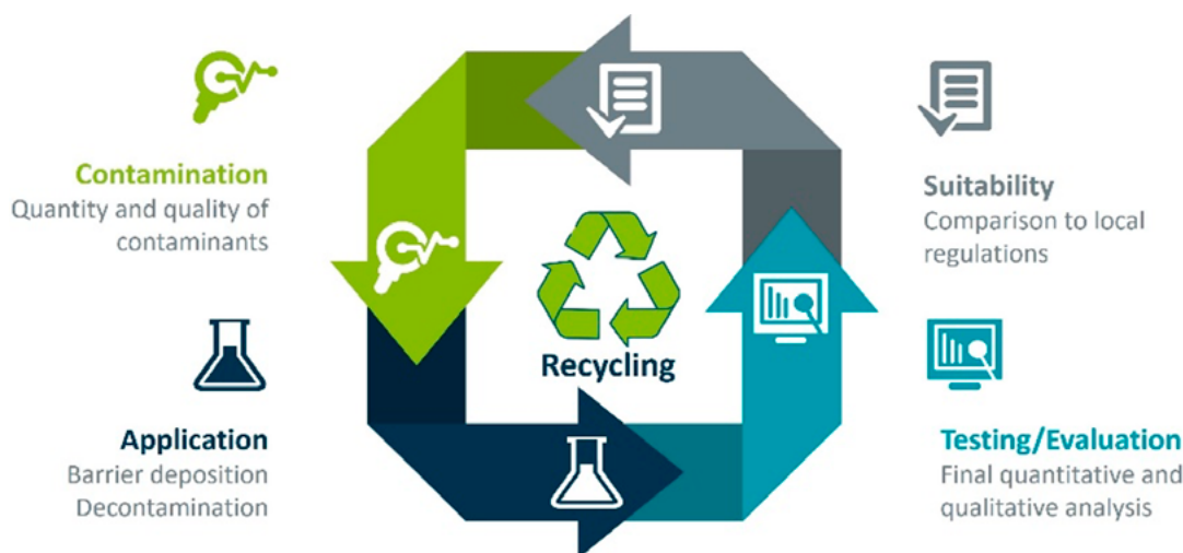
Figure 1. Analytical assessment to determine recyclate suitability.
