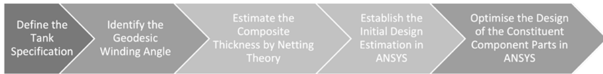
Figure 5. Type IV hydrogen pressure vessel design methodology followed in the work.
