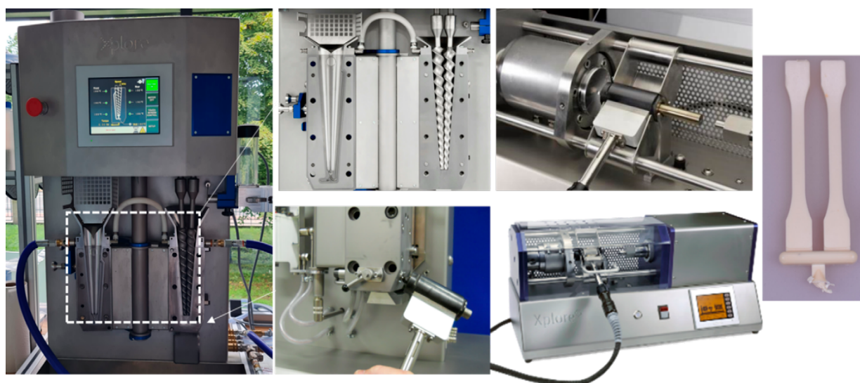
Figure 2. Micro-compounding machine and injection molding setup used for preparation of hybrid filler/PBAT/PLA bio-composites [9].
