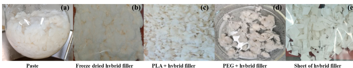
Figure 4. Hybrid filler dosing in different form (a) paste dosing (b) freeze dried filler dosing (c) hybrid filler dissolved in PLA (d) hybrid filler dissolved in PEG (e) sheet dosing.
