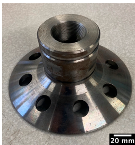
Figure 2. Example of a 316 stainless steel tank boss.
