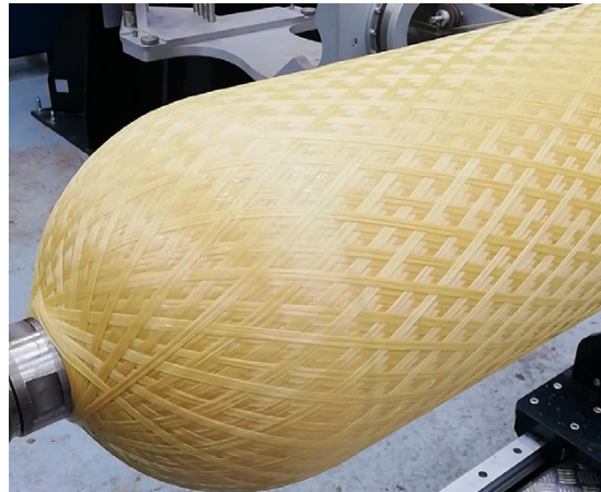
Figure 4. Example of a filament wound Type IV hydrogen tank.
